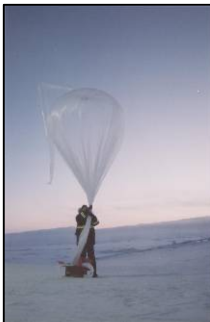
Figure 2: Preparing to launch an ozondesonde. (Photo by G. Nott.)
