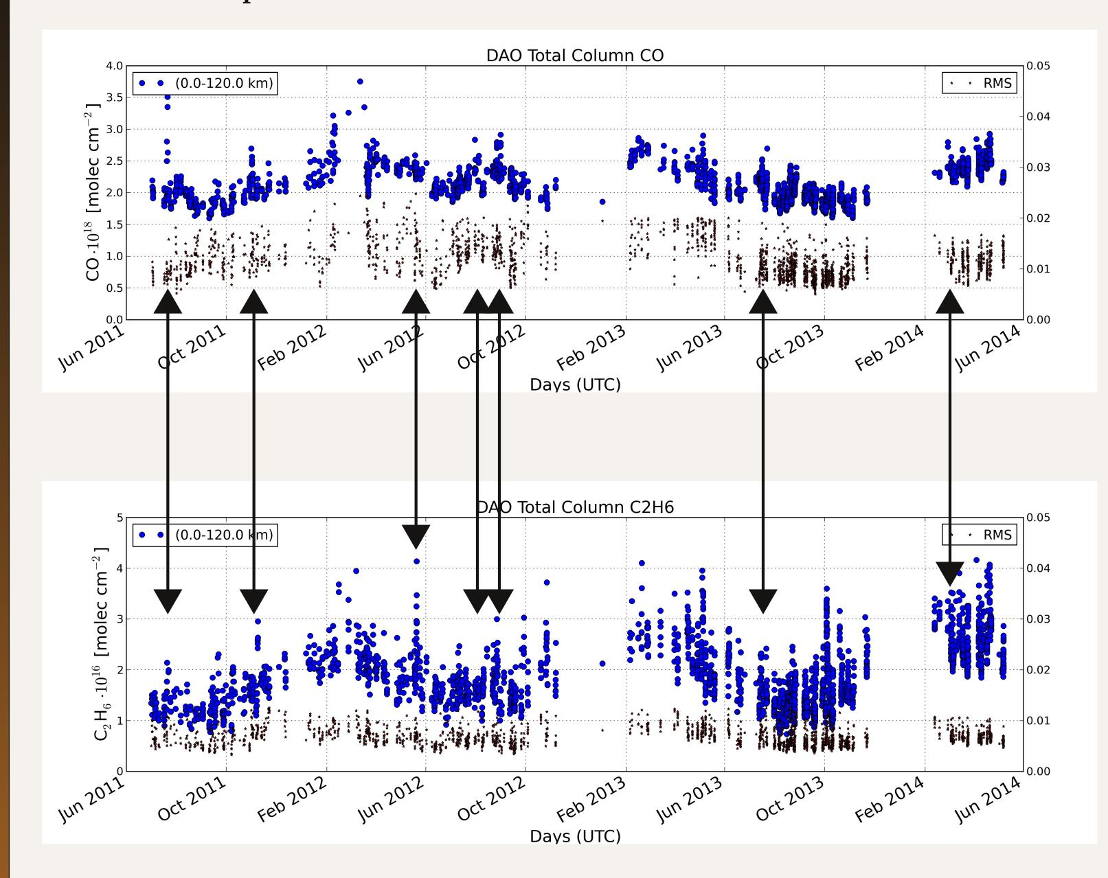
The DAO-DA8 is co-located with a CIMEL sun photometer that is part of the AEROCAN network. The marked points above correspond to enhancements in the CO record that are associated with elevated levels of finemode aerosol optical depth.
