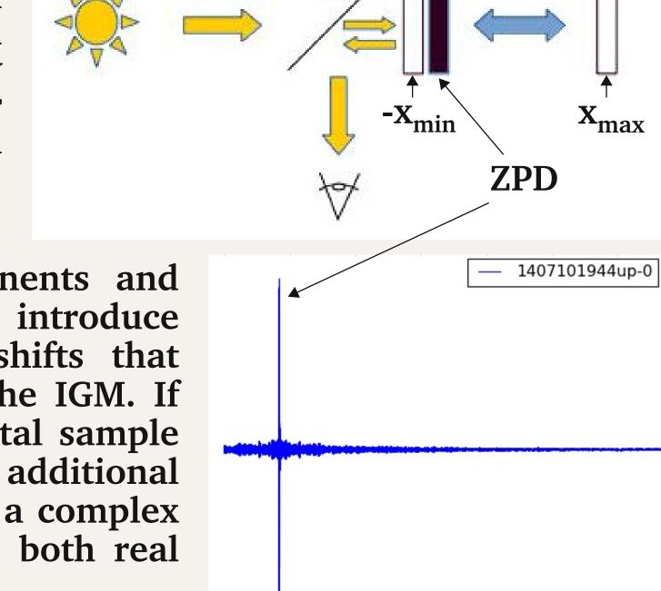
In reality, optical components and sampling electronics can introduce wavelength-dependent phase shifts that will result in asymmetries in the IGM. If the ZPD falls between two digital sample points, this will introduce an additional linear phase shift. In this case a complex Fourier transform will produce both real and imaginary components.
