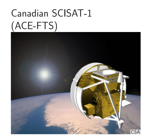
Spaceborne Fourier Transform Spectrometer (FTS) since 2003 [2]. Orbit 650 km, 74°. Solar occultation geometry gives high Signal to Noise Ratio (SNR) and high vertical resolution, but relatively few measurements. Covers  $750 \, \text{cm}^{-1}$ – $4400 \, \text{cm}^{-1}$  $(13.3 \, \mu \text{m} - 2.273 \, \mu \text{m})$  with resolution of  $0.02 \,\mathrm{cm}^{-1}$ . Present study uses version 3.5
