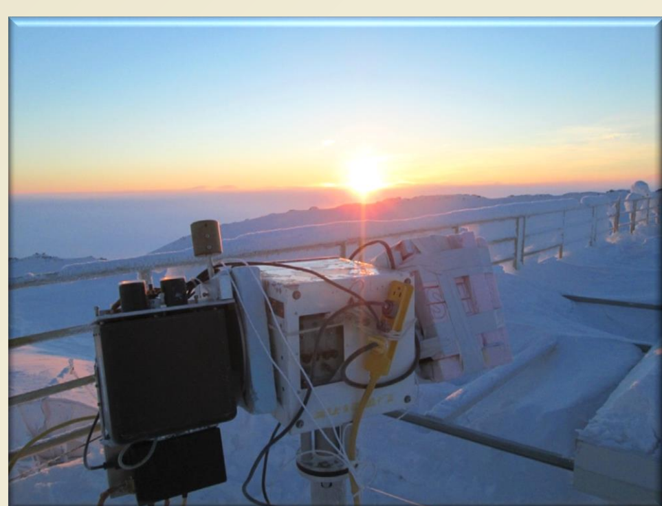
SPS (right) and MAESTRO (left) mounted on a sun-tracker at PEARL station in Eureka, Canada
