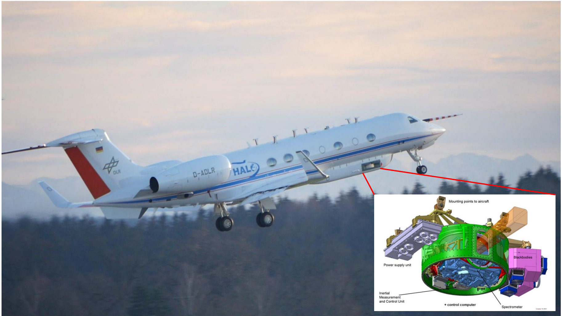
Gimballed Limb Observer for Radiance Imaging of the Atmosphere (GLORIA)
