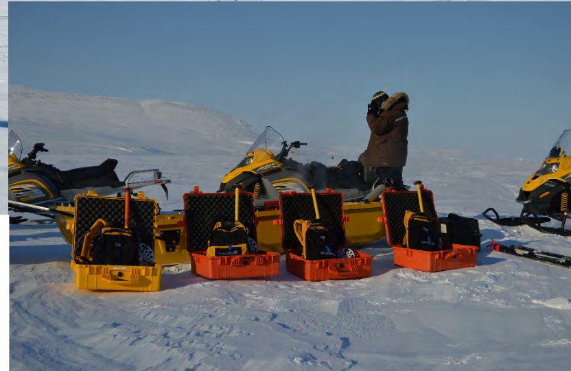
Eureka Sound, Ellesmere Island, NU: Magna probe – snow depth survey using automated GPS-tagged snow depth probes. photo credit: Peter Toose
