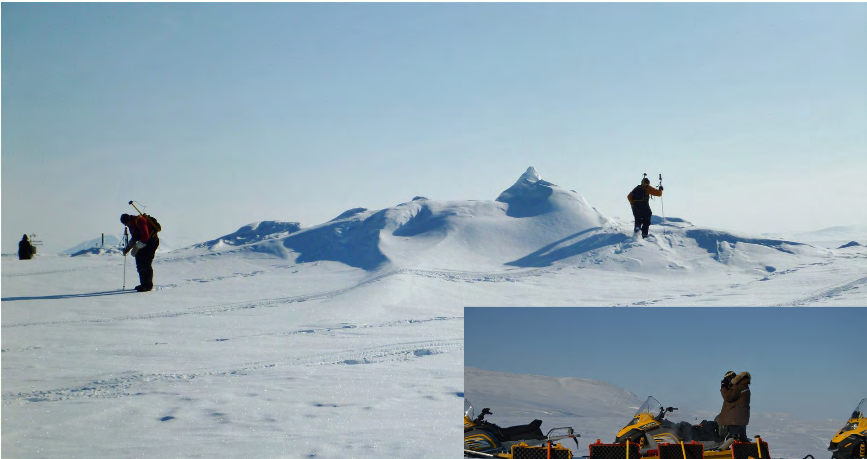
Eureka Sound, Ellesmere Island, NU: Magna probe – snow depth survey using automated GPS-tagged snow depth probes. photo credit: Peter Toose
